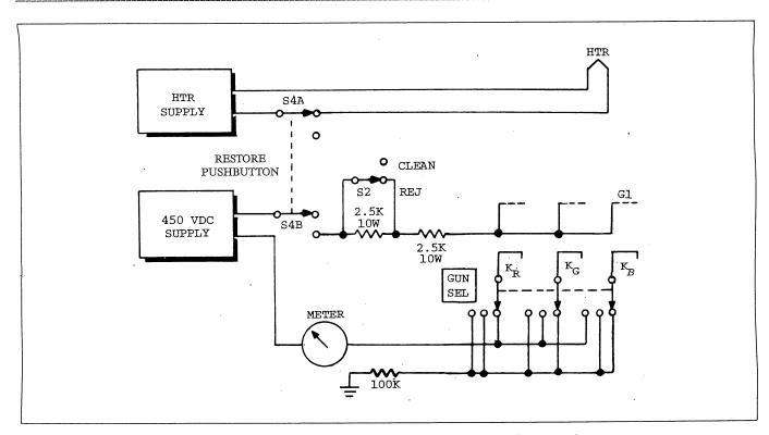
Fig. 6. Model 480 clean, balance, and rejuvenate circuit (simplified).
